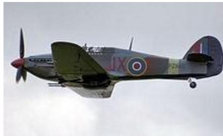
The Hurricane. (The first Hurricanes sent to France during the winter of 1939/40 had 2-bladed propellers. They were replaced by the three bladed version before the "Battle of Britain" started. Metal, instead of fabric covered wings were also introduced)
